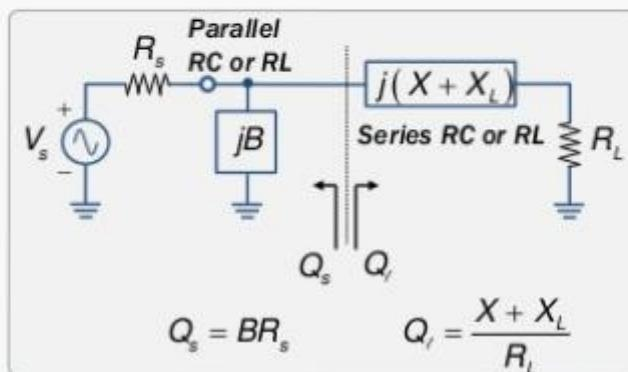
**Imaginary part:**  $(X + X_L) - BR_s R_L = 0 \quad \frac{X + X_L}{R_L} = Q_r = BR_s = Q_s = Q$
